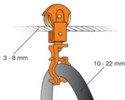
The REMA RKL round cable trolleys are suitable for guiding round cables for the energy supply over a wire rope.
