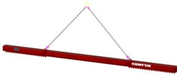
The lifting beam of the T-K-SL series has a 2-strand chain suspension for single hooks according to DIN 15401 on the crane side and shackle bars on the load side. The matching shackles are included in the scope of delivery. You are able to expand the lifting beam with additional equipment from our web shop. The lifting beam is supplied in the standard color RAL 3000 (flame red), other colors are also possible on request.
