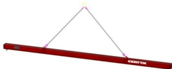
The lifting beam of the T-K-SB series has a 2-strand chain suspension for single hooks according to DIN 15401 on the crane side and rigid shackle plates on the load side. The matching shackles are included in the scope of delivery. You are able to expand the lifting beam with additional equipment from our web shop. The lifting beam is supplied in the standard color RAL 3000 (flame red), other colors are also possible on request.
